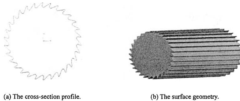
Fig. 5. Surface geometry of plain milling cutter with helix angle.
