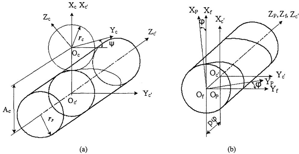
Fig. 2. Coordinate systems applied for the helical milling cutter by disk-shaped tool.
