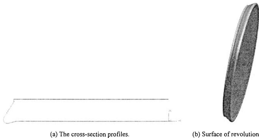
Fig. 6. Surface geometry of form grinding wheel.
