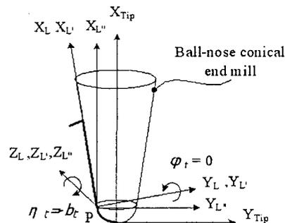
Fig. 4. Coordinate systems of the ball-nose conical end mill.
