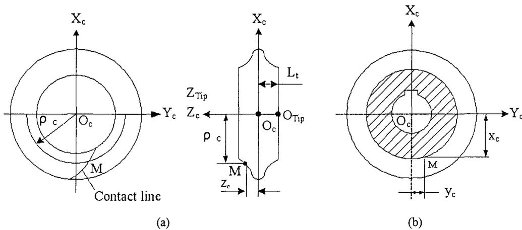
Fig. 3. Schematic illustration of the cross-section profiles of form cutter.
