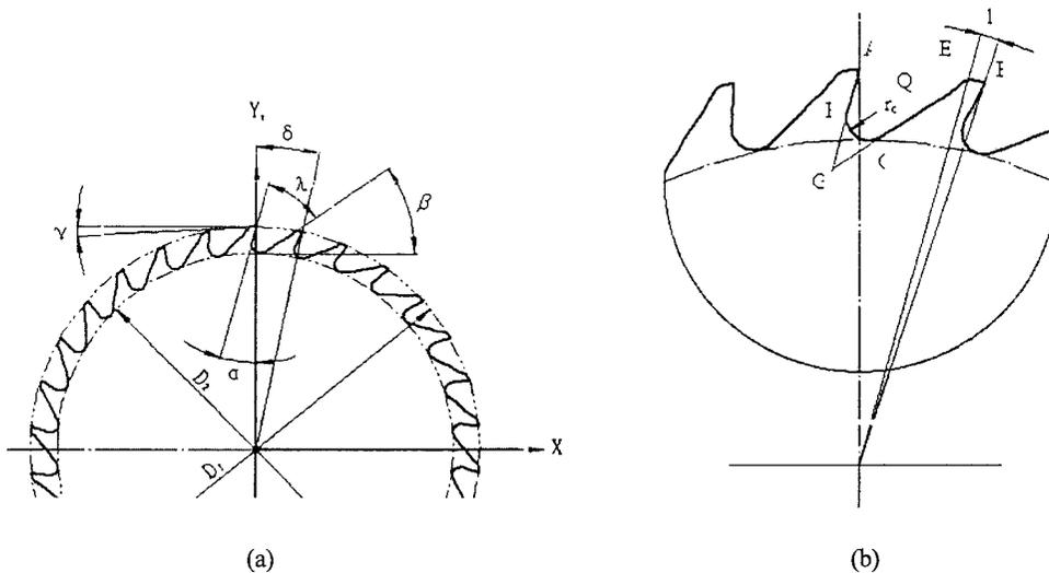
Fig. 1. The cross-section profile of a plain milling cutter with helix angle.
